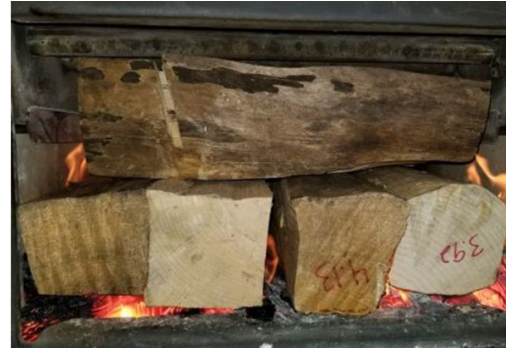
As shown in this photo from a certification test report, the cord wood used by testing labs did not always comply with shape requirements.
